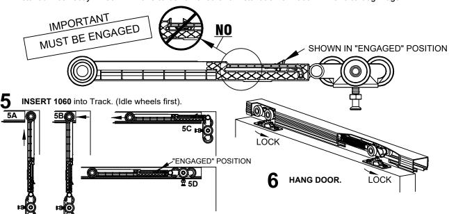
**SLIDE** door away from end of track (check to make sure all track screws are flat against track and does not interfere with movement of dampener hanger) and install 1060 Actuator Arm into track, with back of Actuator Arm 2-1/4" (57mm)
