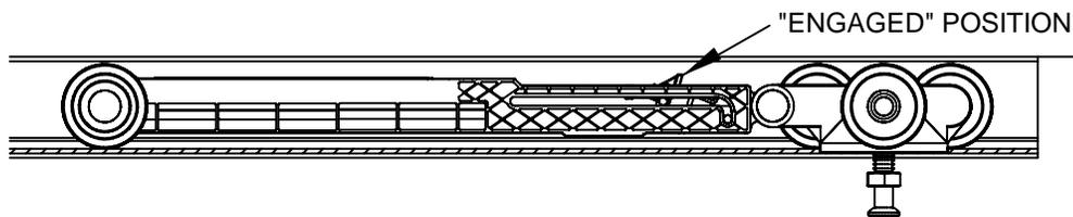
**6** INSERT 1060 Actuator Arm into track, with back of Actuator Arm 1-1/2" (38mm) from end of track, (18-24" doors: Actuator would be flush with end of track). **HAND TIGHTEN** (do not use power drill) Actuator Arm on track legs. Check to make sure Arm remains straight in track.
