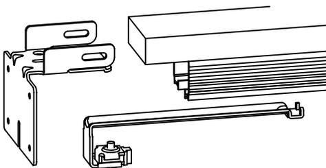
Remove Bracket, Install Actuator Arm, Reattach Bracket.
