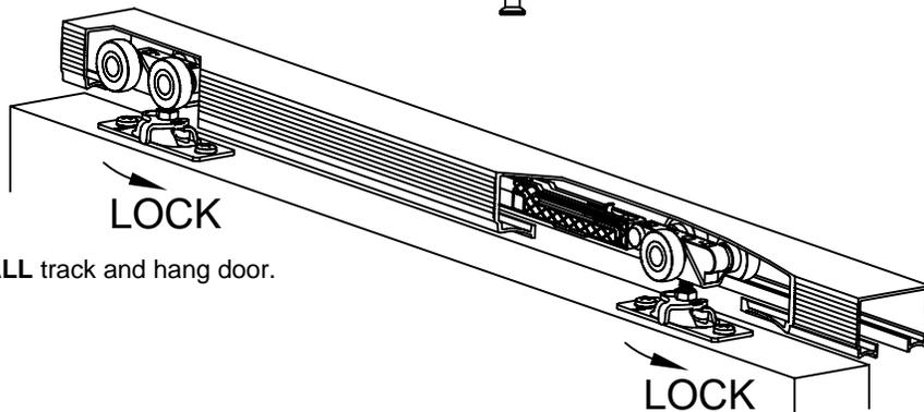
**8** **SLOWLY** slide door toward Jamb, checking to make sure door touches Jamb, if not. Slide door away from Jamb and readjust Actuator Arm. Slowly close door again, checking to make sure soft close is working properly. Once confirmed, begin using door normally.
