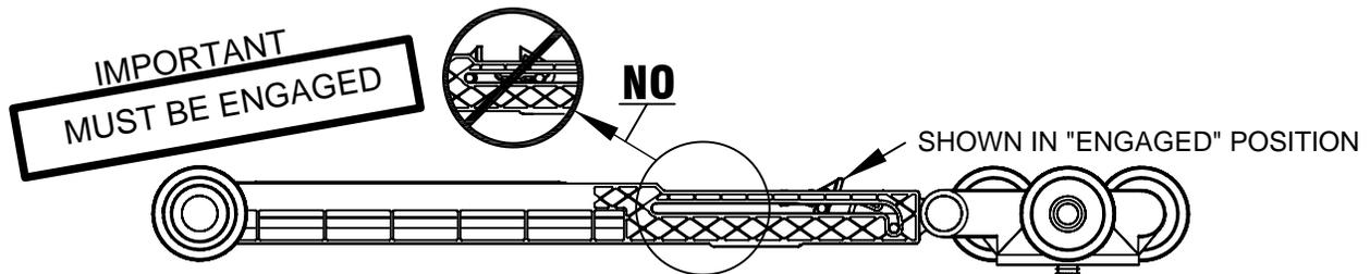
**5** INSERT 1060 into Track. (Idle wheels first).
