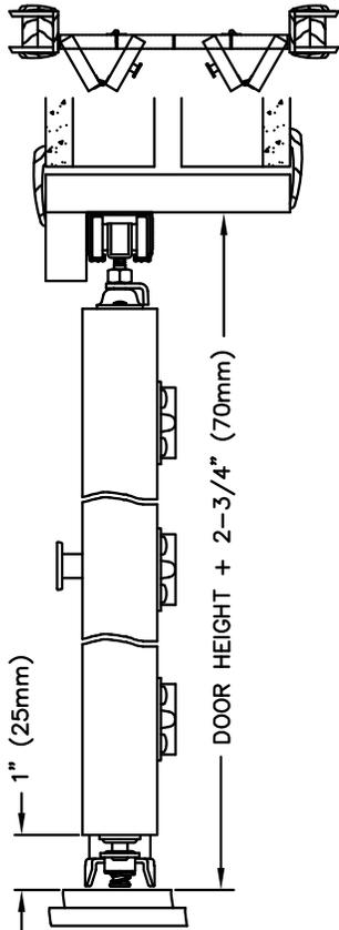
A deluxe commercial grade, folding door hardware set designed for use with heavy 3/4" to 1 3/4" doors weighing up to 50 lbs. per door panel.
