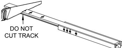
**3** Turn Header over and cut Track 1-3/8" (19mm) shorter than wood Header.
