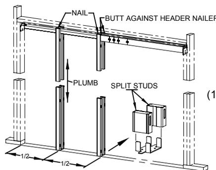
**4** Slip fingers on floor Plates into the reinforcing strips of Split Studs as shown. Butt Split Studs against header nailer strips and nail in place.
