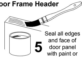
**5** Seal all edges and face of door panel with paint or sealing stain.
