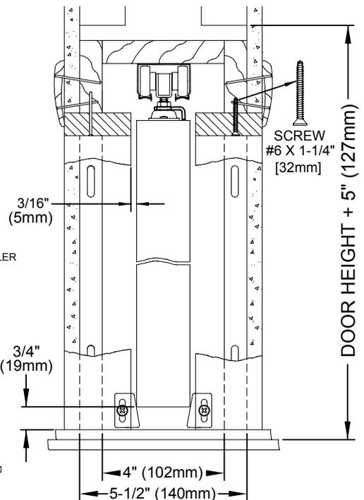
**8** Fasten #1550 Guides on finished split jambs at door bottom so door is held in center of opening without binding.
