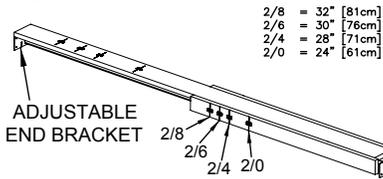
**2** Cut through WOOD part of header only, on desired door size marking.
