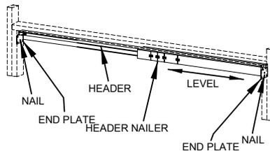
**3** Slip slots in Frame Header End Plates over nails in side jambs.
