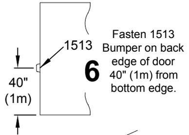
**6** Fasten 1513 Bumper on back edge of door 40" (1m) from bottom edge.
