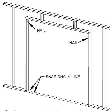
**2** Snap two chalk lines on floor even with side jambs as shown.
