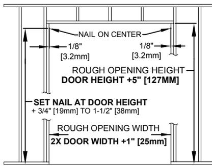
**1** Header must be SQUARE and PLUMB with studs and LEVEL.
