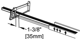
**4** Replace Adjustable End Bracket on new cut end of header.
