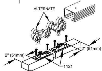
**7** Attach door plate 1121 to top of door 2" (50mm) from each edge with locking tabs on same side. Insert hanger 1125 onto track. Mount door by locating door plate 1121 under adjusting bolt of 1125. Lift door and push bolt into door plate. Lock locking tab.
