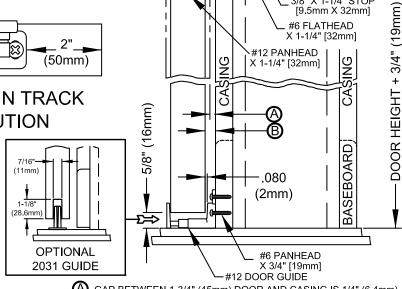
(A) GAP BETWEEN 1-3/4" (45mm) DOOR AND CASING IS 1/4" (6.4mm)
