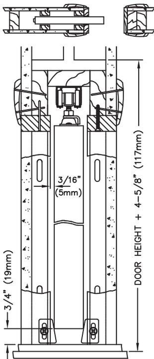
For 2 x 4 Construction. Removable aluminum track with convex rails for smooth quiet operation, rust resistant steel reinforced wood split studs, jump proof three wheel (3/4" dia.) hangers, self adjusting floor anchors, 2'6" and 3'0" headers marked to cut to smaller door sizes. Brass-tone steel parts. All frames for doors up to 1 3/8" can be converted for 1 3/4" doors with 1575PPK3 adaptor kit. Very similar to 1500 Series Frame, but with smaller diameter hanger.
