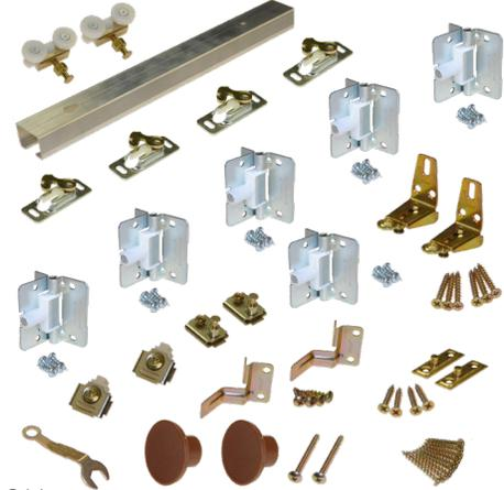
A superior light commercial bifold hardware set for 12"-24" panels up to 9' high weighing 50 lbs. each. Convex rail aluminum track with positive pivot lock, top hung, three wheel (3/4" dia.) hangers, four-way adjustable jamb bracket, shock absorbing "breathing" hinges self locate and automatically align to door. Brass-tone steel parts.
