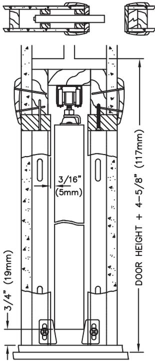
For 2 x 4 Construction. Removable aluminum track with convex rails for smooth quiet operation, rust resistant steel reinforced wood split studs, jump proof three wheel (1" dia.) hangers, self adjusting floor anchors, 2'6" and 3'0" headers marked to cut to smaller door sizes. Brass-tone steel parts. All frames for doors up to 1 3/8" can be converted for 1 3/4" doors with 1575PPK3 adaptor kit.
