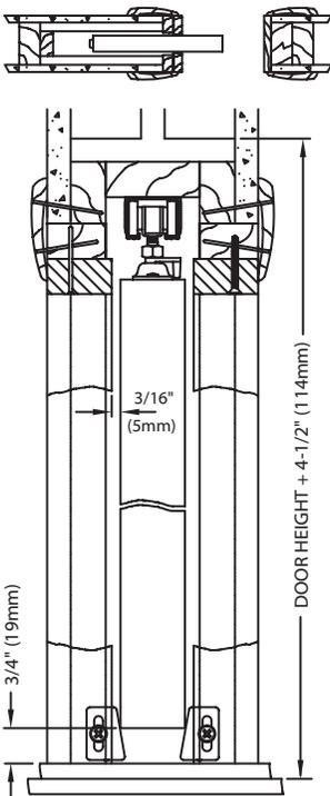
A "pre-assembled" pocket door frame with 10 horizontal members for 2" x 4" construction. Removable aluminum track with convex rails, jump proof three wheel (3/4" dia.) hangers. Brass-tone steel parts. *Optional hanger #1025 available for doors to 150 lbs.*
