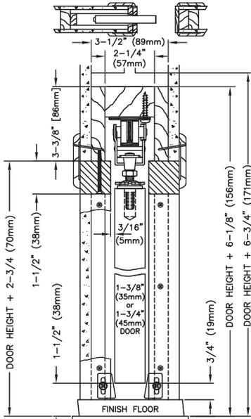
For 2 x 4 construction. Aluminum "I" Beam track, smooth quiet operation, rust resistant all steel split studs, jump proof 4 wheel ball bearing (1" dia.) hangers, self-adjusting floor anchors, 2'6" and 3'0" headers marked to cut to smaller door sizes. Plated steel parts. Now comes with the 2041 hidden guide set.
