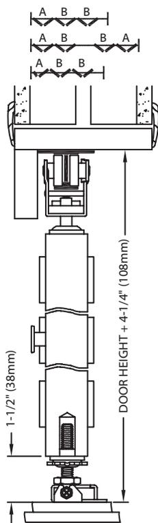
Hardware for panels 12"-36" up to 9'0" high. Heavy duty I-beam track with positive pivot-lock, top hung, four wheel (1" dia.) ball bearing hangers, heavy duty bottom pivot, floor bracket with screw adjusting bottom pivot socket. Plated steel parts.
