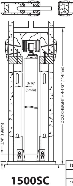
For 2 x 4 Construction. Same features as the 1500 Series frame, but it includes two 1060 soft close assemblies to enable both soft close and soft open along with the smooth rolling of ball-bearing hangers. Now come standard with the new All-Steel Studs. More rigid and works for 1 3/4" thick doors right out of the box. No Adapter needed.
