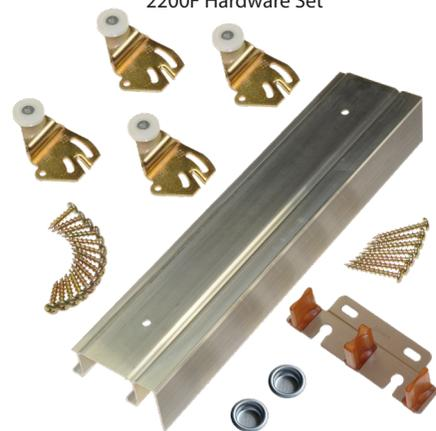
An aluminum fascia track with "Hi-Lite" design to hide blemishes that may occur. Convex track rails that provide one point contact between wheel and track. Hangers include one or two wheels (7/8" dia.) with three point locking. Hangers adjust without removing or relocating screws. Woodtone guide adjusts laterally for quick plumbing. Nylon guide posts are 1" high, guide posts swivel to allow warped doors to operate without binding. Brass-tone steel parts.
