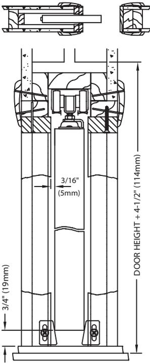
A "pre-assembled" pocket door frame with 10 horizontal members for 2" x 4" construction. Removable aluminum track with convex rails, jump proof three wheel (1" dia.) hangers. Brass-tone steel parts. *Optional hanger #1125 available for doors to 200 lbs.*
