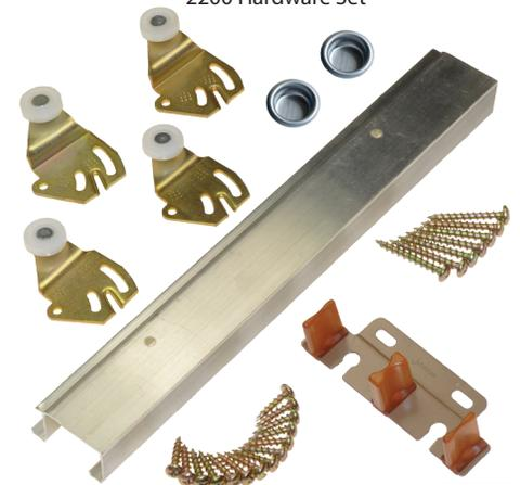
Aluminum bypass track with convex track rails for quiet, smooth operation. One wheel (7/8" dia.) hangers with three point locking provide one point contact between wheel and track. One inch high woodtone adjustable door guide. Brass-tone steel parts.
