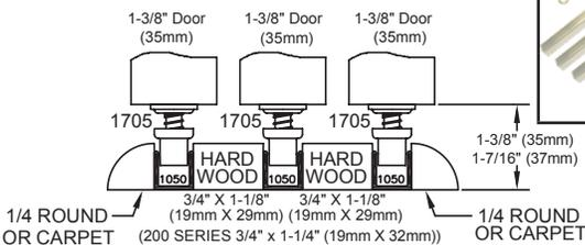
All nosing and hardware filler supplied by others. Surface mount shown/ Bottom channel may be recessed into floor. Spacing and dimensions will vary with other door thicknesses.
