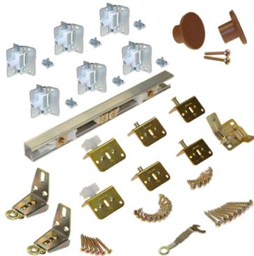
Same features as 170A series, except hardware is mounted to back side of door. Side mount plates can be adjusted if opening is slightly out of square. Top pivot and guide must be kept parallel with track. Track also available in white and brown.
