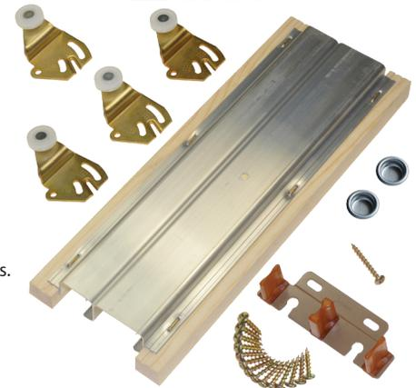
Prefabricated header with aluminum track replaces the regular head jamb. Keeps the bypass doors the same trim height as swinging doors. Eliminates odd door heights. Convex track rails, 7/8" dia. wheels, adjustable hangers, adjustable guide. Brass-tone steel parts. Also available for 5/4" jamb and without wood. Contact factory.
