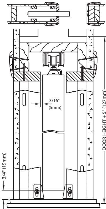
For 2 x 6 Construction. Removable aluminum track with convex rails, rust resistant steel reinforced wood split studs, jump proof three wheel (1" dia.) ball bearing hangers, self-adjusting floor anchors, headers marked to cut to smaller door sizes. Brass-tone steel parts.
