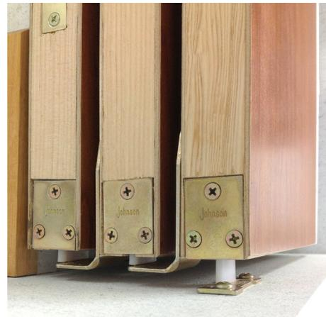
Side mount guide posts can be used to allow for a setup that does not require bottom guide tracks. Individual guide posts are used and travel inside a groove in the bottom of each door to make for a clean floor in the opening.
