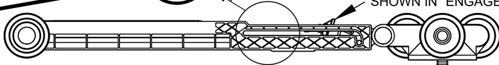
**5** INSERT 1060 into Track. (Idle wheels first).
