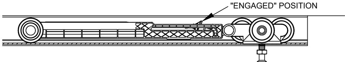
**5** INSERT 1060 Actuator Arm into track, with back of Actuator Arm 1-1/2" (38mm) from each end of track, (24" doors: Actuator will be flush with end of track). **HAND TIGHTEN** (do not use power drill) Actuator Arm on track legs. Check to make sure Arm remains straight in track.
