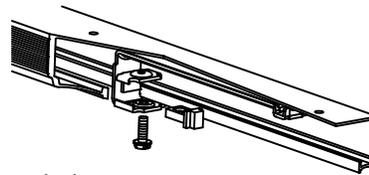
**4** IF NEW INSTALLATION insert Actuator Arm as shown below.
