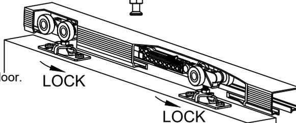
**8** SLOWLY slide door toward Jamb, checking to make sure door touches Jamb, if not. Slide door away from Jamb and readjust Actuator Arm. Slowly close door again, checking to make sure soft close is working properly. Once confirmed, begin using door normally.
