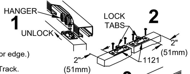
**2** ATTACH 1121 Door Plates 2" (51mm) from door edge. (18-24" Door: Attach Door Plates 1/2" (12.5mm) from door edge.)
