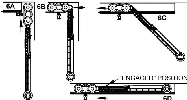
**8** INSERT 1125 Ball Bearing Hanger Wheel assembly into Track.
