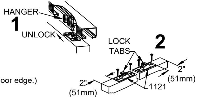
**2** ATTACH 1121 Door Plates 2" (51mm) from door edge. (24" Door: Attach 1121 Door Plates 1/2" (12.5mm) from door edge.)
