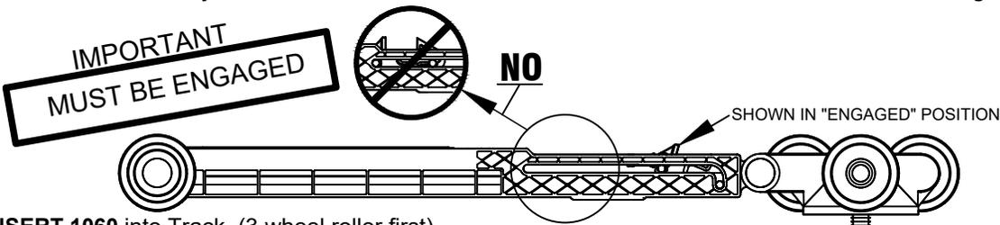
**7** INSERT 1060 into Track. (3 wheel roller first).
