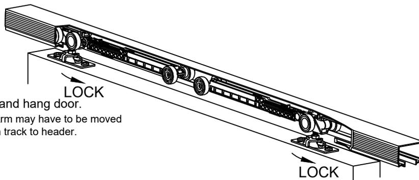
**SLOWLY** slide door toward Jamb, checking to make sure door touches Jamb, if not. Slide door away from Jamb and readjust Actuator Arm. Slowly close door again, checking to make sure soft close is working properly. Once confirmed, begin using door normally.
