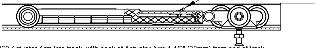
**6** INSERT 1060 Actuator Arm into track, with back of Actuator Arm 1-1/2" (38mm) from end of track, (18-24" doors: Actuator would be flush with end of track). **HAND TIGHTEN** (do not use power drill) Actuator Arm on track legs. Check to make sure Arm remains straight in track.
