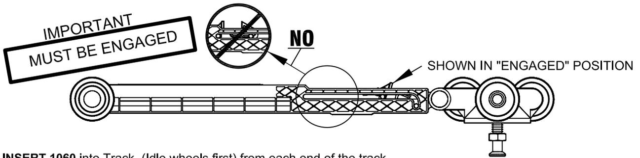
**4** INSERT 1060 into Track. (Idle wheels first) from each end of the track.
