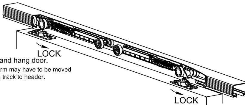
**SLOWLY** slide door toward Jambs, checking to make sure door touches Jamb, if not. Slide door away from Jamb and readjust Actuator Arm. Slowly close door again, checking to make sure soft close is working properly. Once confirmed, begin using door normally.
