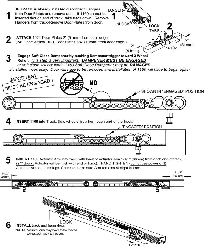
**SLOWLY** slide door toward Jambs, checking to make sure door touches Jamb, if not. Slide door away from Jamb and readjust Actuator Arm. Slowly close door again, checking to make sure soft close is working properly. Once confirmed, begin using door normally.
