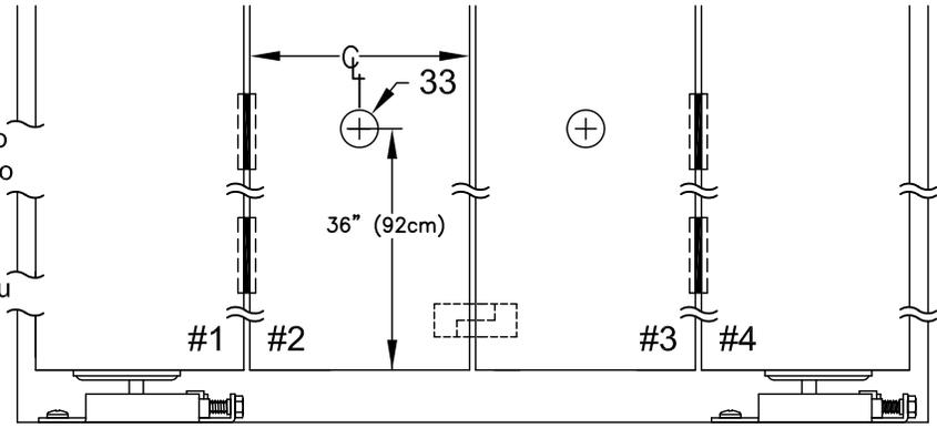
**9 ADJUST SNUBBER (1155)** Close doors, slide 1155 until it touches 1125. Open doors, move 1155 1/8" (3mm) closer to 1125 and tighten.
