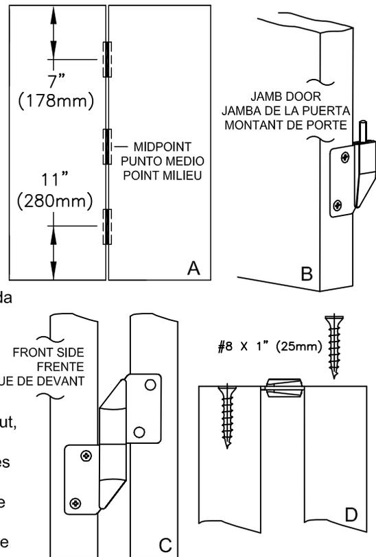
**3 FASTEN PIVOT PLATES** to top and bottom of doors as shown. Note: 1121 nylon locking arm must open towards rear of opening.
