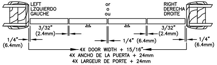
**PREPARE OPENING CAREFULLY: MAKE SURE CORNERS ARE SQUARE, HEADER IS LEVEL AND JAMBS ARE STRAIGHT**
