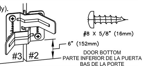
**7 CHECK FOR PROPER DOOR OPERATION:** clearance, alignment, adjustment, etc. should be made at this time. If adjustments are required, they can be made at Track Pivot Socket 1010 and Floor Bracket 1011. Settling, door warpage and other uncontrollable conditions may require later adjustments. **Note: Doors must be parallel with track for proper operations.**
