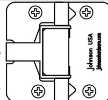
**3 FASTEN PIVOT PLATES** to top and bottom of doors as shown.
