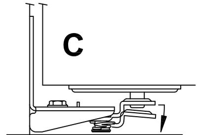
**7 ADJUST SNUBBER (1713)** Close doors, slide 1713 until it touches 1705. Open doors, move 1713 1/8" (3mm) closer to 1705 and tighten. Doors should "snap" shut yet open easily by a slight pull on the knob.
