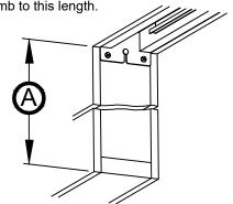
**2 OPEN** door fully (door will protrude into opening) and cut split jambs to "B" Fasten to front edge of frame. Maintain minimum 3/16" (4.7mm) clearance on both sides of door. Raise or lower hangers to plumb door with split jambs.
