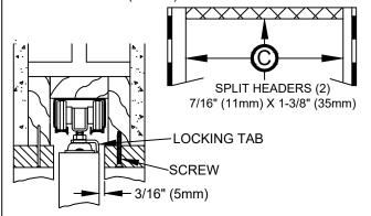
**5 FASTEN** bottom door guides so that door stays in center of pocket, yet travels easily without binding.
