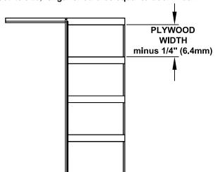
**3** ATTACH Plywood Clip Brackets as shown to each piece of plywood using 3/4"(19mm) x #6 Pan Head Screws.
