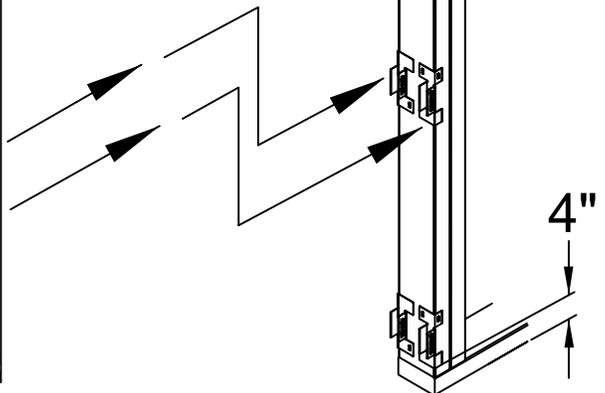
**6** **SLIP** Fingers of Floor Bracket into a pair of split studs, butt Split Stud against plywood sheets making sure split studs go into 1515 bracket attached to the plywood sheets. Nail split studs to header, plumb studs, nail to floor between chalk lines.
