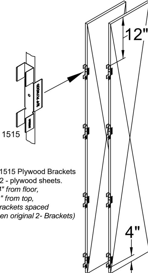
**4** **ATTACH** 4 - 1515 Plywood Brackets to one end of 2 - plywood sheets.
