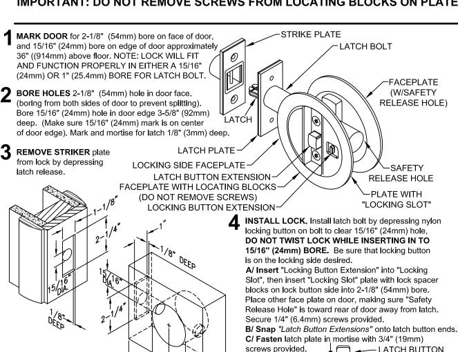
**INSTALL STRIKER.** Slide pocket door closed, hitting jamb to mark location. Drill 15/16" (24mm) hole 1" (25.4mm) deep in center of marks made by latch. Place strike plate in 15/16" (24mm) hole, making sure plate is plumb with jamb, then mark and mortise, 1/8" (3mm) deep. Secure with 3/4" (19mm) screws provided.
