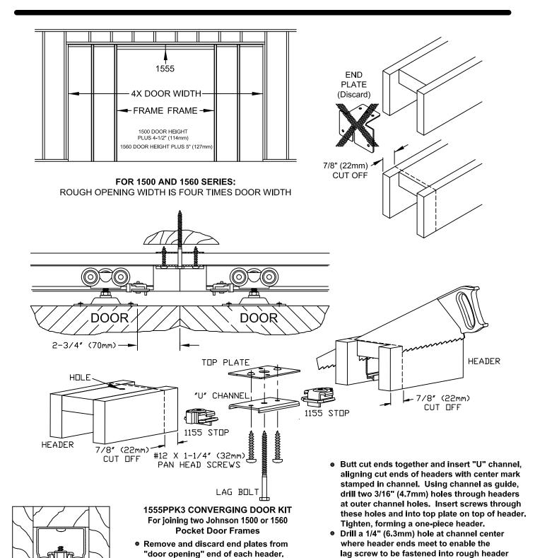
• Cut 7/8" (22mm) from length of each header
