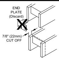
1556PLBG CONVERGING DOOR KIT For joining two Johnson 1562 Pocket Door Frames
