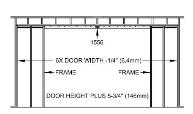
ROUGH OPENING WIDTH IS SIX TIMES DOOR WIDTH -1/4" (6.4mm)
