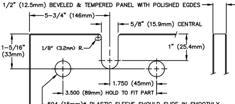
**1 HAVE GLASS** beveled, drilled and tempered per illustration.
