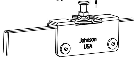
**7 HANG GLASS DOOR.** Adjust Hanger then tighten locknut.
