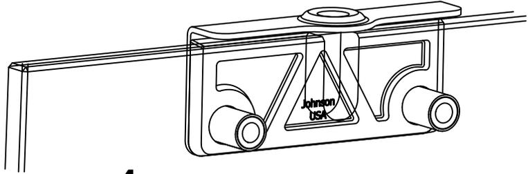
**4 INSERT DOOR PLATE** into holes drilled in door.
