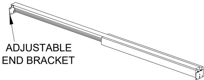
**5** Replace Adjustable End Bracket on new cut end of header.
