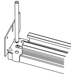
**3** Cut through WOOD part of header only at mark.
