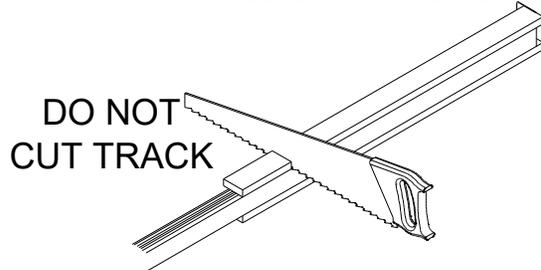
**4** Turn Header over and cut Track 1-3/8" shorter than wood Header.
