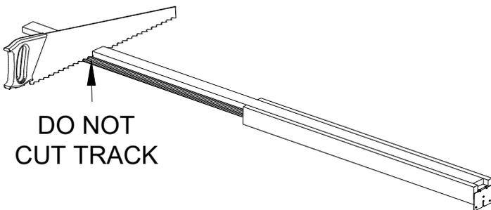
**6** Turn Header on side and cut Side Nailer Trim Board ONLY at mark. Remove cut off end and discard.
