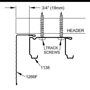
Install track as shown in diagram at left, 3/4" (19mm) from front edge of header. Fasten track loosely with #8 X 1-1/4" (32mm) screws. Slip FASCIA between track and header so that beaded edge locates in track groove as shown at left. Tighten track screws to snug FASCIA to header. If required, additional screws (not supplied) may be used to provide additional FASCIA security.
