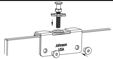
**6 LAY OTHER HANGER PLATE** against pad and thread 3/8" screws into metal post. Thread hex slotted Locknut onto adjusting bolt, then thread adjusting bolt into door plate.
