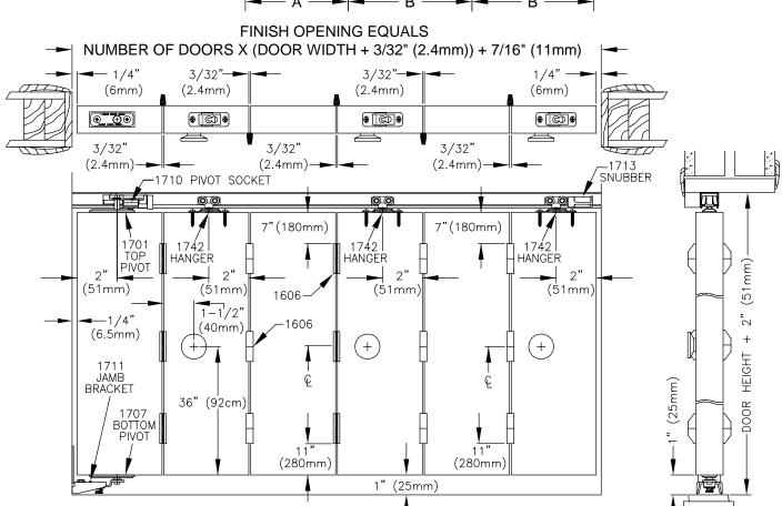
CUT TRACK TO LENGTH. Insert pivots, hangers and snubber as required. Fasten track to center of top header. Locate 1710 Pivot Socket in proper position and fasten in place. Unlock pivot socket by moving lock tab away from jamb.
