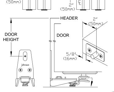
HANG rest of doors by dropping door down over hinge in preceeding panel. Clip hangers in place on respective doors.
